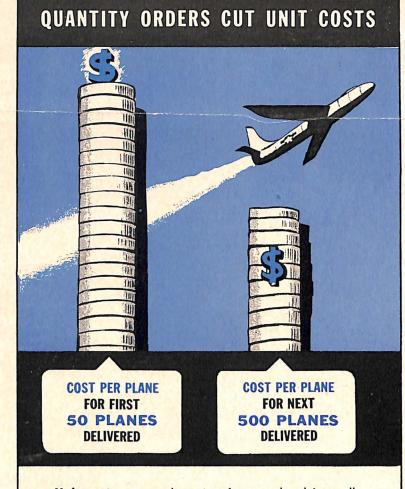
Unit costs go up when aircraft are ordered in small quantities—and go down when they are produced in substantial volume. Typical of savings being realized by the military services through quantity orders is the case of a modern jet plane now being flown by the Air Force. The first 50 planes cost approximately 65 per cent more per unit than did the following 500.
