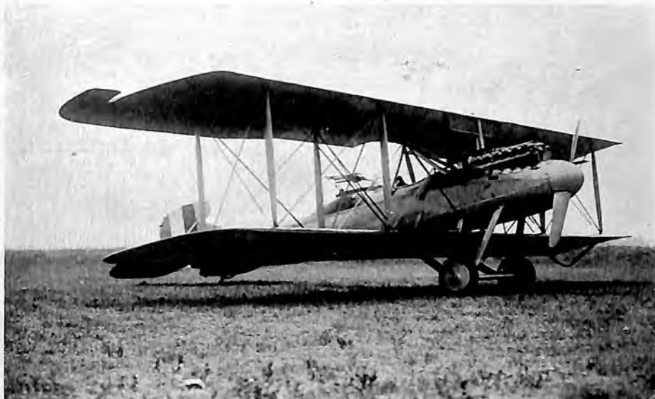
Model G, the first L-W-F Plane which flew with the Liberty 12-Cylinder Motor
