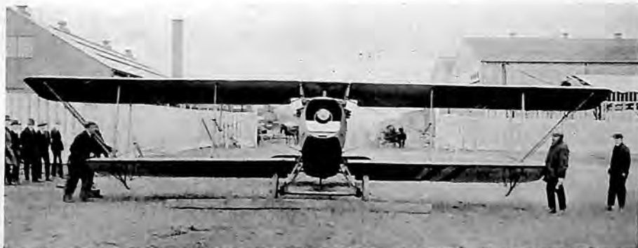
Model E-4. This is identical with JR-1-B, except for overhang. It mounts a 150 H. P. Hispano-Suiza Engine
