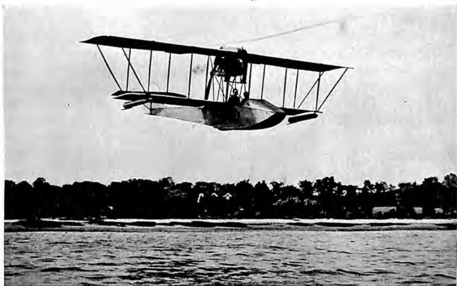
Model B Flying Boat (steel hull) making a flight
