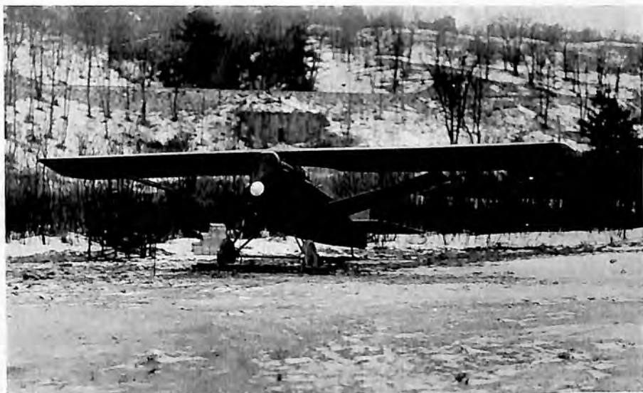
M-B-1 Fighter, Two-Place, with 450 H. P. Liberty Engine
