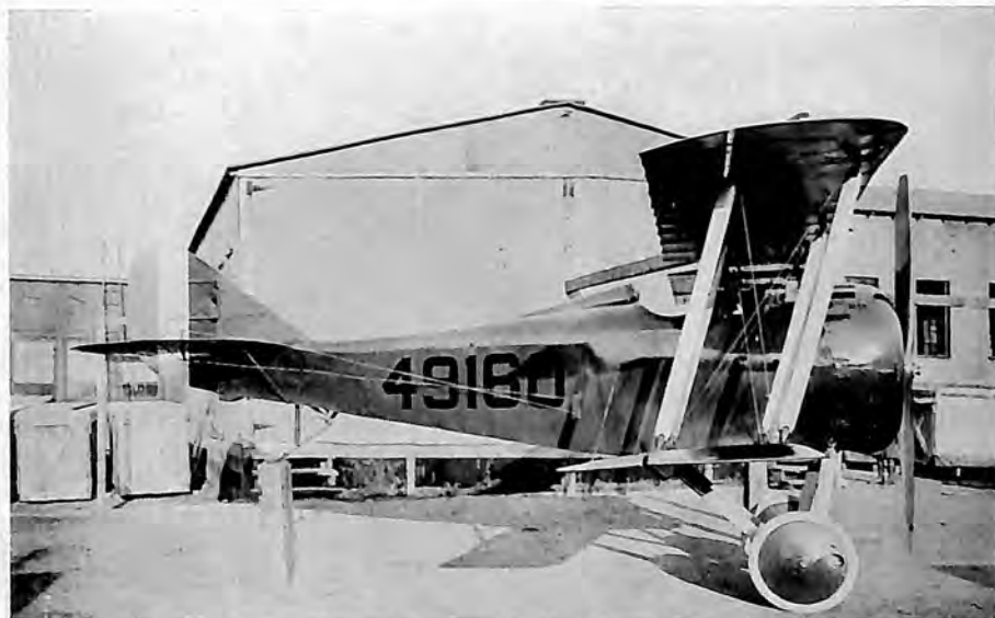
Model E-1—a defense advance training Tractor Aeroplane, single-seater with a 100 H.P. 9-Cylinder Rotary Gnome Engine
