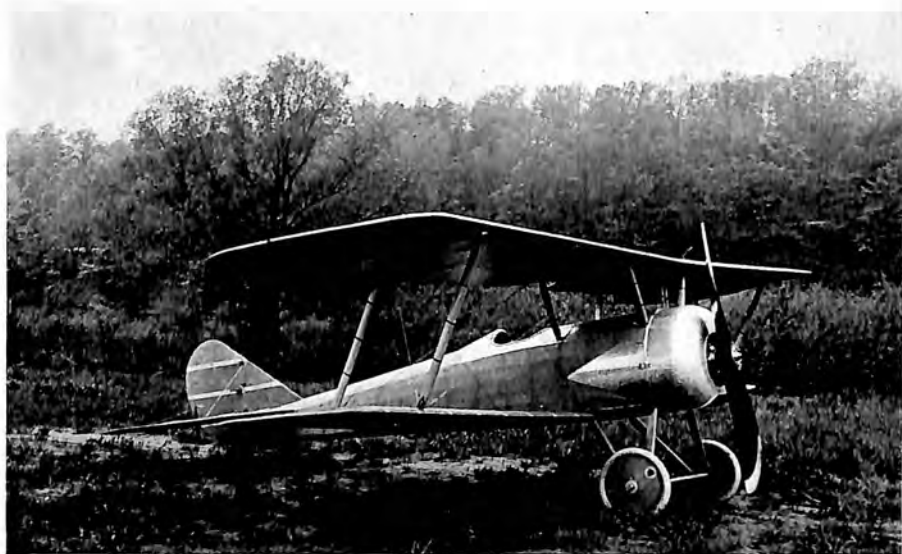
S-4 Scout, One-Place, with 100 H. P. Gnome Engine
