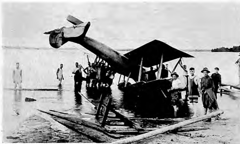
The same Machine after the hurricane. The fuselage, it will be seen, is still in good condition
