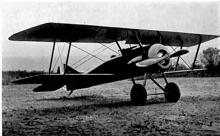
S-4-C Scout Type, with 80 H. P. LeRhône Engine
