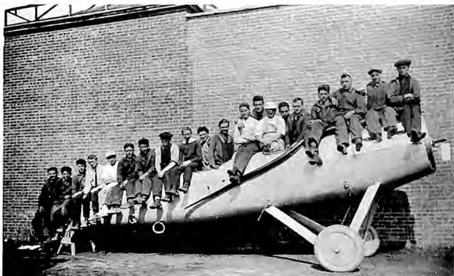
An L-W-F Fuselage for Model V. Note the twenty men which the shell supports
