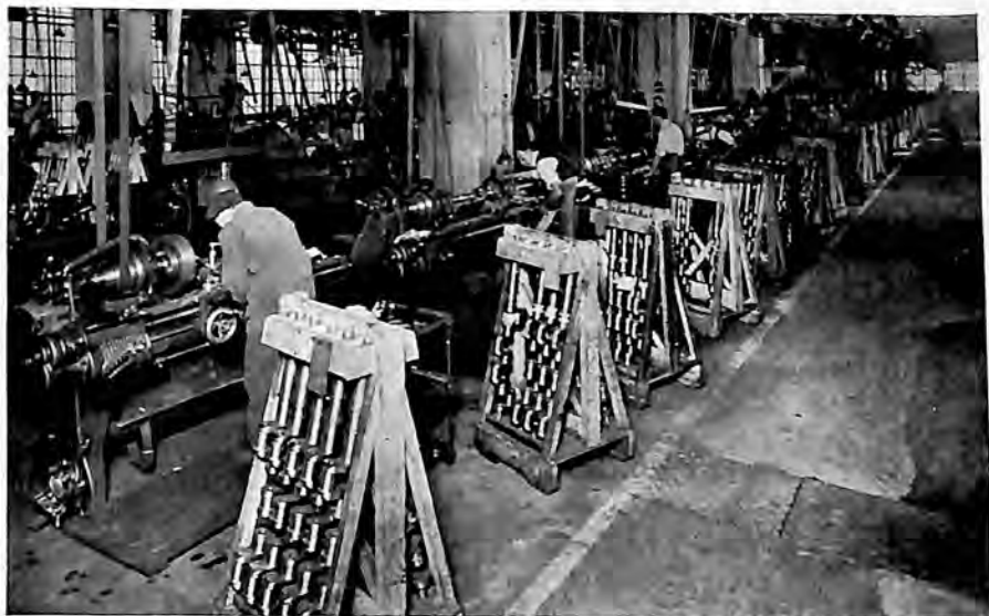
Crankshaft Line in the New Brunswick Factory, exclusively devoted to the 150 and 180 H. P. Motors
